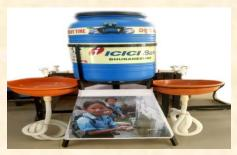
water source at the tube-well point or at the pipe source point has been introduced with little expenditure of a plastic pipe, few taps and if required a rubber pipe. With the help of this rubber pipe the multi-tap water source can
